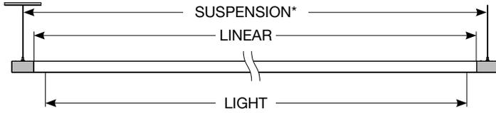
\*Suspension points are calculated between a STRAIGHT STARTER FEED and END SEGMENT/JOINER. For all other configurations, refer to component dimensions below.
