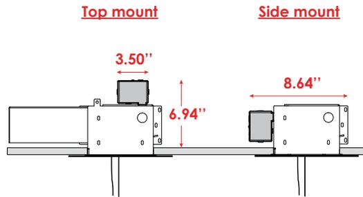
\*Mounted on standard 4" octagonal j-box. Fits on any j-box with 5/8" knockouts
