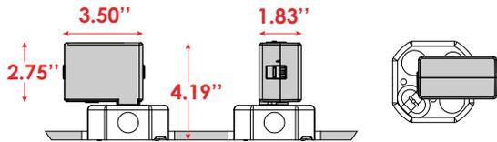
\*Mounted on standard 4" octagonal j-box. Fits on any j-box with 5/8" knockouts
