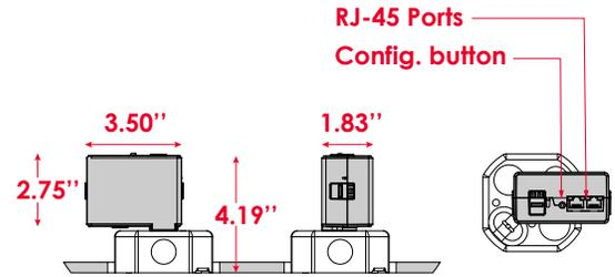
\*Mounted on standard 4" octagonal j-box. Fits on any j-box with 5/8" knockouts
